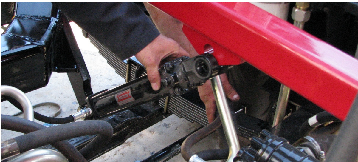
Install the provided T Booster hydraulic cylinder, attaching to the Mil-Stak mounting bar and T Booster.
